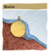
Wattles create a dam-like structure that causes water to back up and flow over the top, resulting in potentially severe erosion on the down slope side of the wattle.
