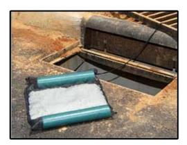
Dandy Skimmer is used to combat oil contamination. Measuring 22" x 14" x 2", this uniquely designed screen pillow is filled with a polymer absorbent that has not one but two attached flotation devices. The oil absorbent material inside the skimmer easily captures the oil - permanently and continuously.
