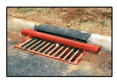
With an open-top design, the Dandy Curb Sack fits to any size curb and gutter inlet. Its unique design allows it to filter sediment-laden water with ease. The suspended solids are allowed to settle out of the slowed flow and are captured quickly by the Dandy Curb Sack before entering the inlet.
