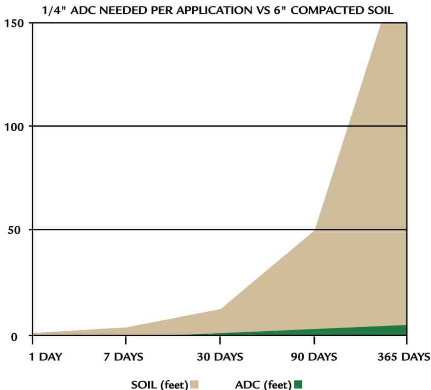
Chart demonstrates amount of landfill space lost over the course of a year with a standard soil application compared to ADC. ADC requires minimal coverage of 1/4-inch per application, resulting in greater available landfill space for waste.
